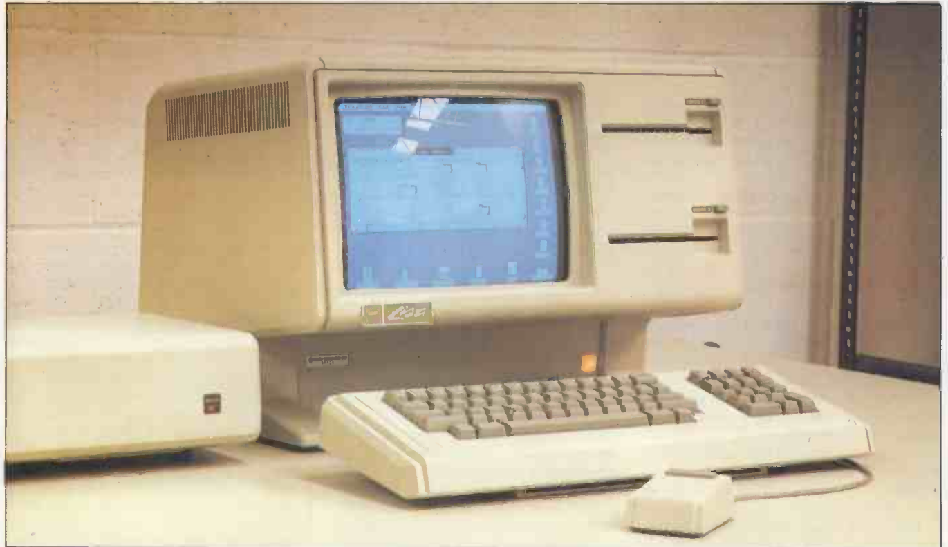
The system unit is compact, incorporating 12in screen on the left and storage for the keyboard underneath.
