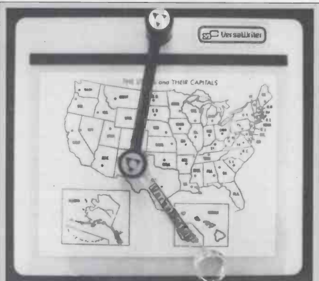
Looking like a glass elbow over a map, the Versawriter connects to the IBM micro as a way of feeding drawings into the computer memory. It costs £200, and is available from Pete & Pam on (0706) 212321.
